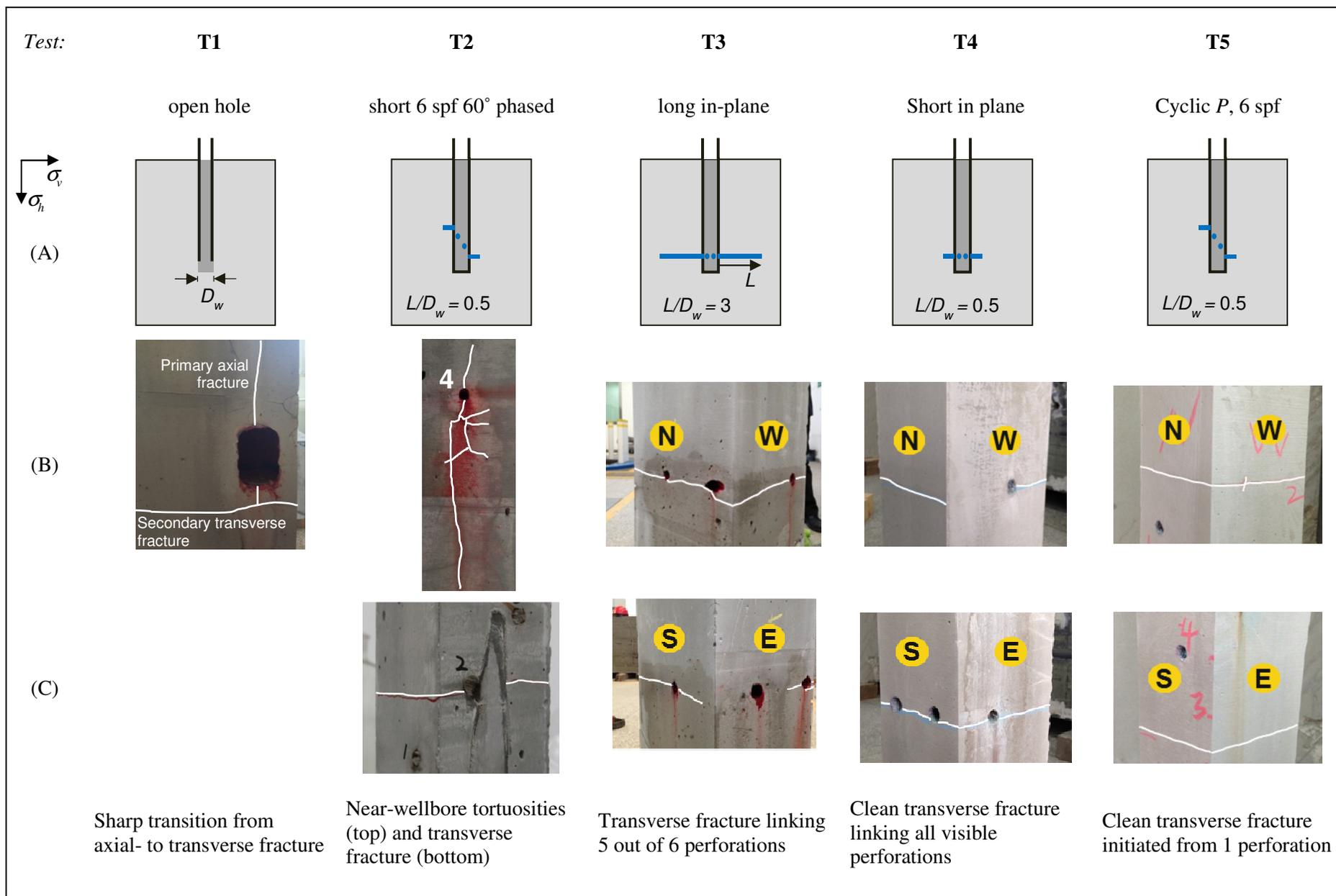
Fig. 5: Completion geometries (A) and their respective near-wellbore fracture geometries (B-C).
