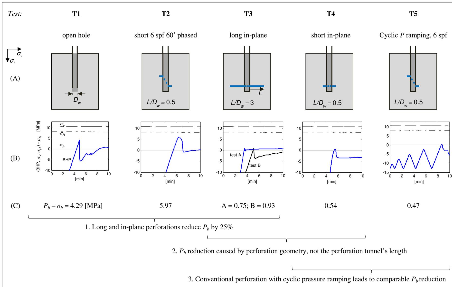
Fig. 4: Completion geometries (A) and their respective pressure curves (B) with normalised breakdown pressure  $P_b$  (C).
