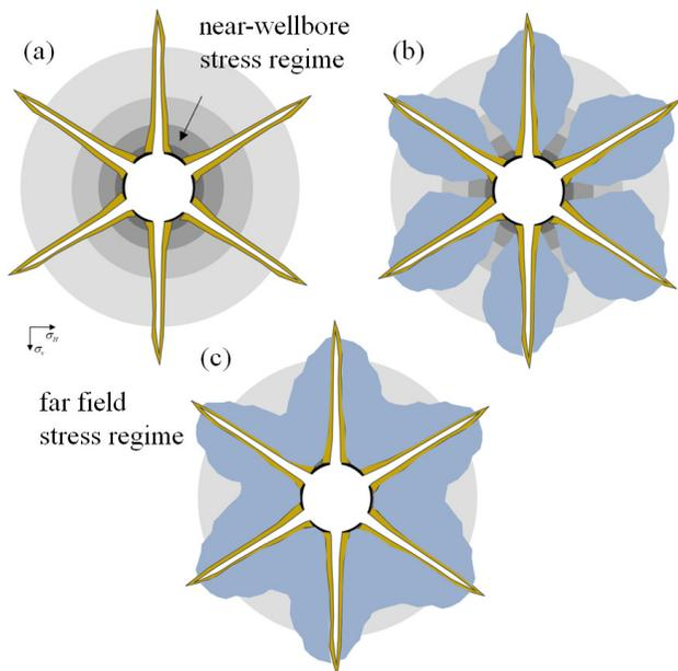
Fig. 3: schematics of: in-plane perforations penetrating into the far field stress regime (a); hoop-stress failure of perforation tunnels initiating fractures in a single plane (b); circumferential linking up of fractures, merging into a single transverse fracture (c).
