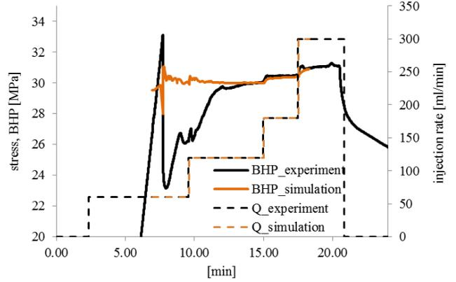
Fig. 9: Numerical simulation of the open hole experiment (T1).
