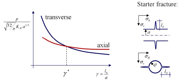
Fig. 2: theoretical fracture reorientation criterion (left) with the hypothetical starter notch configurations (right) [7].
