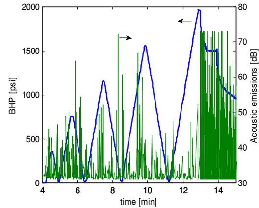
Fig. 7: Acoustic emissions (green) during the cyclic pressure ramping (blue)
