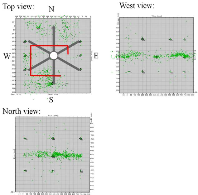
Fig. 6: Acoustic events with respect to the perforation tunnel orientation (grey) and the continuous circumferential fracture (red).
