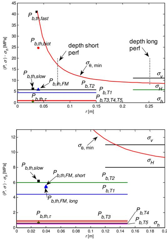
Fig. 8: Actual breakdown pressures of T1 – T5 in comparison with the theoretical models in equations (1) – (4);  $\sigma_h$ -normalised principal stresses  $\sigma_v$ ,  $\sigma_H$ , and the minimum hoop stress  $\sigma_\theta$ . The bottom figure is a zoomed-in view of the top figure.
