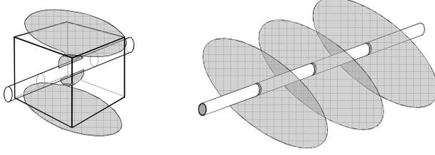
Fig. 1: Undesirable fracture tortuosities: caused by the transition between near-wellbore and far field stress regime (left); transverse fractures reaching from the wellbore into the far field (right).
