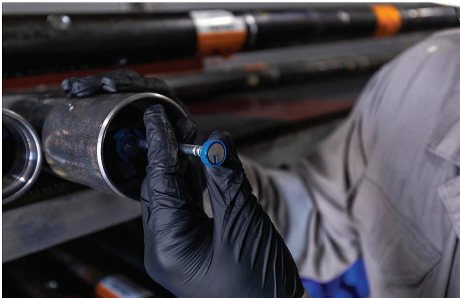
We designed a detonator system that greatly reduces the chance of mishaps, misruns and misfires. We coupled it with the DynaStage perforating gun, which is fully factory-assembled and requires no wiring at the wellsite. There are no electrical or ballistic connections to be made. The only procedure is to install the simple plug-and-go detonator into the gun, test and run downhole.
